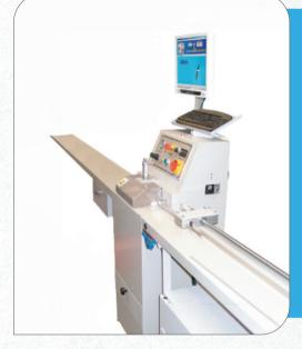
The Computerised Bar Cutter has been designed to utilise sealed unit batch data, either by disk or as part of a network. The saw is accurate, fast and safe to operate with the bar stop moving automatically to the particular highlighted size. The bars are pushed to the stop and with footpedal activation, clamped and cut in one operation. Batches can be uninterrupted and the saw used in manual operations at any time. The saw is designed for use with spacer and Georgian Bar Grills.
