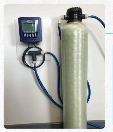
Using a readily available mixed bed ion exchange resin with our pressure vessel and meter is probably the simplest method of producing very pure water for your glass washing needs. Mains water is able to percolate through the resin before being monitored by an accurate conductivity meter before entering your machine.
