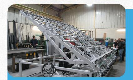
Our Hydraulic Tilting Tables are designed to enable the movement of heavy glass from the vertical to horizontal.
