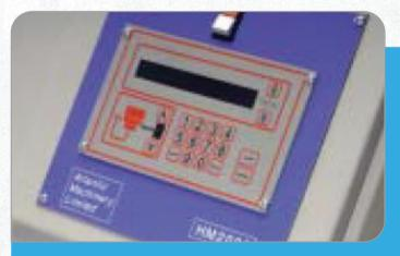
Accurate temperature control is achieved by utilising the latest electronic temperature control coupled with the reliability of Type K thermocouple probes. The larger 'keypad" type machines are pre-calibrated for all the different hot melt sealants, changeable at the press of a button.
