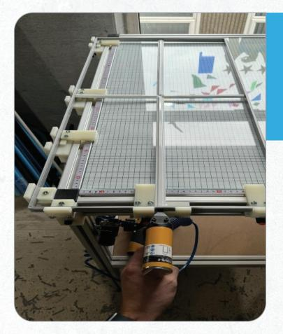
Our Georgian Staple Table is the ideal production aid for Georgian Bar and other specialist internal grills. The table and special clamps allow the frames to be produced perpendicular and the Georgian bar centralised before simply stapling into place.
