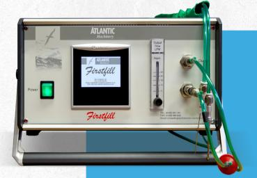
The Firstfill is an introductory gas filler for customers wanting to make low volumes of Argon filled insulated glass units. It has a flow rate of 10 litres a minute and uses the two hole filling method.
