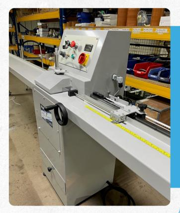
Our Digital Spacer Bar Saw provides a faster, safer and more accurate means of cutting either spacer or georgian bar. The operator can remain in one position adjusting the stop distance with an easy to use wheel and digital display. The clamping and cutting of the bar is then activated by pressing the foot switch, making it impossible for any blade related accidents. Repetitive Georgian cuts can be accurately done using the locking stop and tape for consistency.
