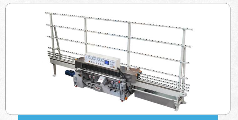
The ASL6.325A 6 spindle edger offers bottom edge and arris grinding and/or polishing depending on the quality of finish required.
