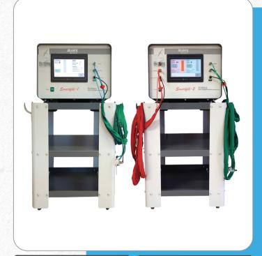
The Smartfill-1 is a single line 30 litre a minute machine designed for the production of Argon gas filled insulated glass units. The Smartfill-1 is the first machine in the Inagas range to be equipped with the unique Smart start lance system which can be used either to gas fill using the one or two hole filling method.
