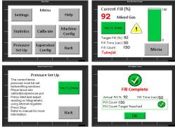
A 100mm touch screen gives a live display of the timed gas filling process and is also used to access the menu screen. From the menu screen gas percentage levels, overfill timer, data logging, pressure set and calibration features can be accessed. A foot pedal switch can be used to remotely start the filling process.
