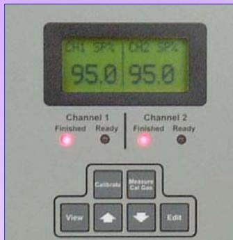
The touch pad controls enables gas percentage levels to be changed, dwell times to be altered, and includes fault finding analysis.
